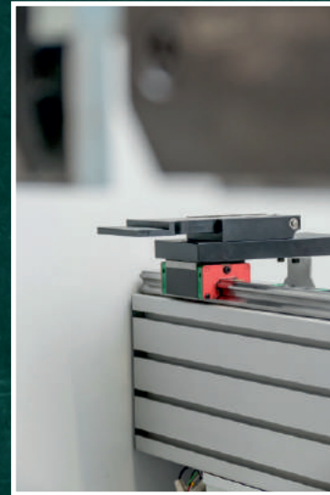
5-axis back gauge - BG5. Axis configuration including Y X, R, Z1, Z2 and Delta X.
